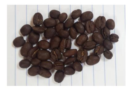
At the factory every destoners is tested. Below is an example of the test material used in the factory tests. Under roasted coffee has been used in the tests alone along with a series of stones to test the performance of each destoner.
