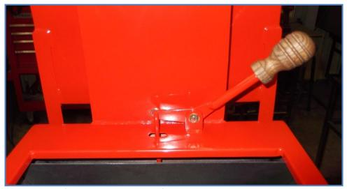
For the best results a few beans will be left behind in the in the spring loaded door at the bottom of the destoner, see the figure below.
