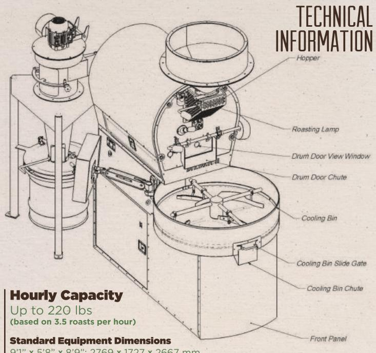
9'1" x 5'8" x 8'9"; 2769 x 1727 x 2667 mm (Overall Dimensions May Vary with Optional Items) Volts AC (1-Phase): 220v/60Hz or 230v/50Hz Single Phase
