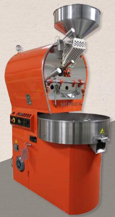
The IR-12 is designed to roast up to approx. 26.4 lbs (12 kg) of green coffee per batch.
